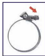
3. Snap screw down and tighten.
