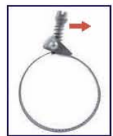
2. Slip band through housing.
